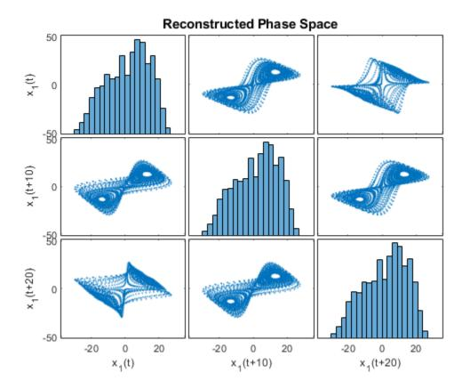
As observed from the 3x3 phase space plot, the topology of the attractor is recovered.  $x_1(t + 10)$  and  $x_1(t + 20)$  are the other two states reconstructed with the estimated lag value of 10. The diagonal plots (1,1), (2,2) and (3,3) represent the histogram of  $x_1(t)$ ,  $x_1(t + 10)$  and  $x_1(t + 20)$  data, respectively.
