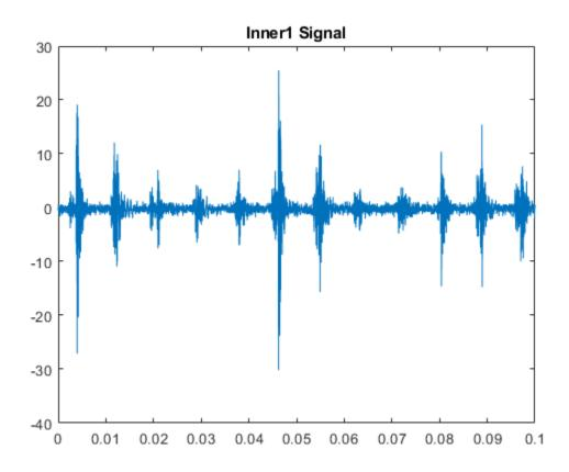
The plot shows periodic impulsive variations in the acceleration measurements over time.
