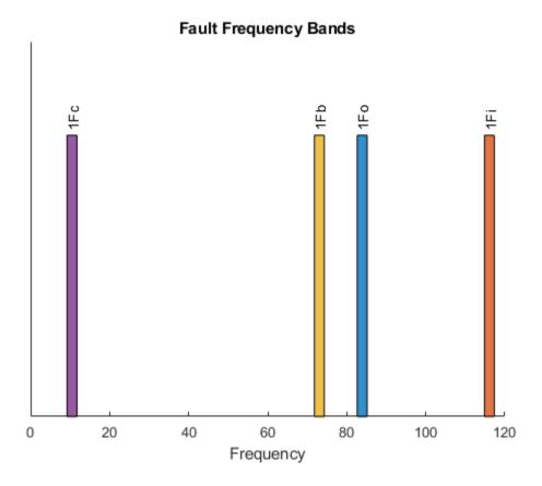
From the plot, observe the following bearing specific vibration frequencies:
