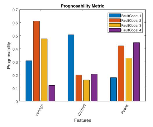
prognosability returns a histogram plot with the features ranked by their prognosability values. A higher prognosability value indicates a more suitable condition indicator. For instance, the candidate feature Current has the highest degree of prognosability for machines with FaultCode 1.
