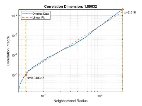
The first dashed, vertical green line (on the left) indicates the value of MinRadius, while the second vertical green line (on the right), represents MaxRadius. The dashed red line indicates the linear fit line for the correlation integral versus neighborhood radius data, within the computed range of radius.
