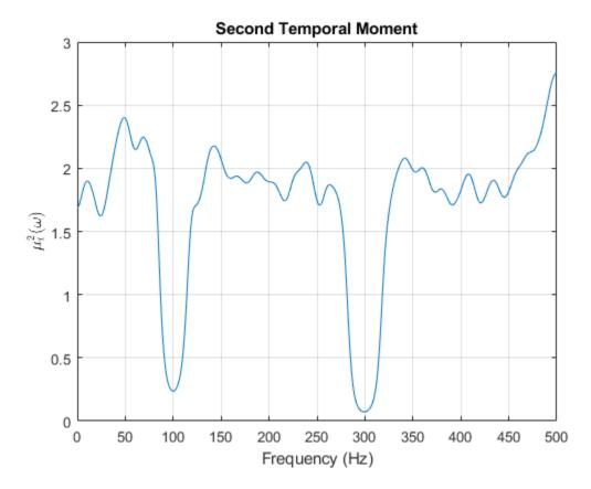
There are two distinct features in the plot at 100 and 300 Hz corresponding to the induced resonances shown by the spectrogram. The moments are much closer in magnitude than the spectral results were.
