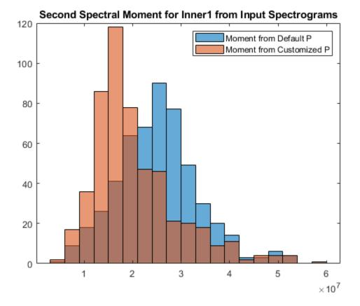
The histograms have the same overall spread, but the thresholded moment histogram has a higher peak bin at a lower moment magnitude level than the default moment. This example is for illustration purposes only, but does show the impact that preprocessing in the spectrum computation stage can have.
