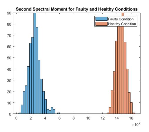
The moment behaviors distinguish the faulty condition from the healthy condition in both plots. The histogram provides distinct distribution characteristics — center point along x-axis, spread, and peak histogram bin.
