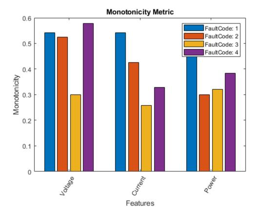
monotonicity returns a histogram plot with the features ranked by their monotonicity values. A higher monotonicity value indicates a more suitable prognostic parameter. For instance, the candidate feature Current has the highest monotonic trend for machines with FaultCode 1.
