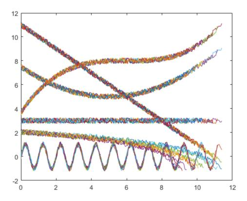
Observe the 6 different condition indicators-constant, linear, quadratic, cubic, logarithmic, and periodic-for all 10 machines on the plot.
