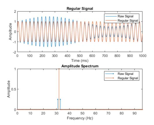
From the plot, observe the waveform and amplitude spectrum of the regular and raw signals, respectively. Observe that the regular signal contains the unmodulated sine wave with an amplitude of 1.0 units and frequency of 32 Hz.
