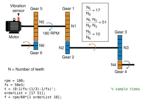
In practice, you would use measured data such as vibration signals obtained from an accelerometer. For this example, generate TSA signal X, which is the simulated data from the vibration sensor mounted on the motor.
