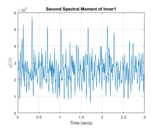
The plot illustrates the changes in the variance of the x\_inner1 spectrum over time. You are limited to this visualization (moment versus time) because tfsmoment returned no data. Now use tfmoment again to compute the second spectral moment, this time using the syntax that returns both the moment values and the associated time vector. You can use the sample rate directly in the syntax (sr\_inner1), rather than the time vector you constructed (t\_inner1).
