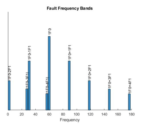
Observe that the sideband frequencies 1F0-3F1 and 1F0-4F1 are now visible on the positive axis.
