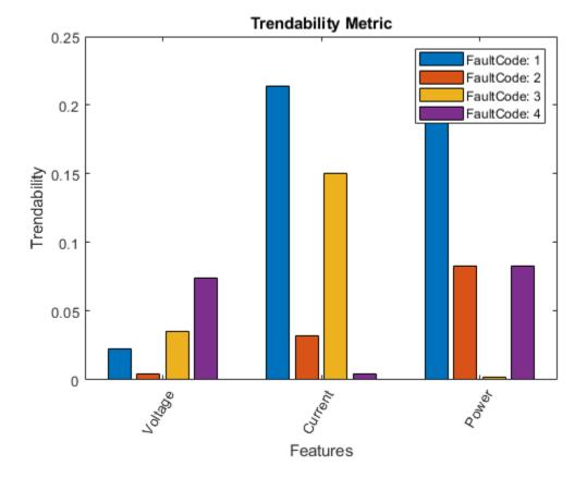
trendability returns a histogram plot with the features ranked by their trendability values. A higher trendability value indicates a more suitable prognostic parameter. For instance, the candidate feature Current has the highest degree of trendability for machines with FaultCode 1.
